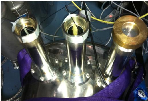
Figure 10. Two outlet bayonets opened
