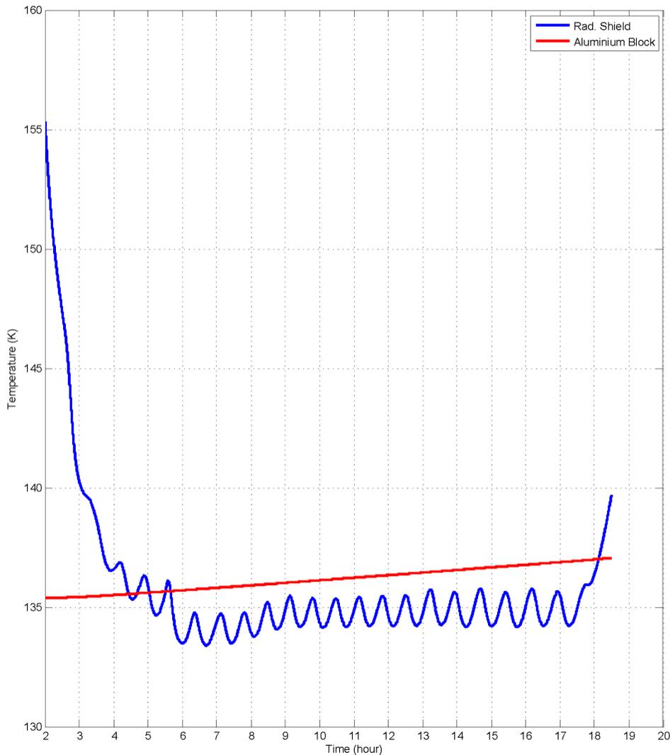
Figure 18. Evolution of the radiation shield and the aluminum block temperature
