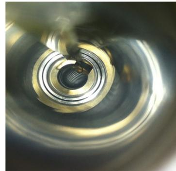
Figure 11. Diode sensor inside the bayonet
