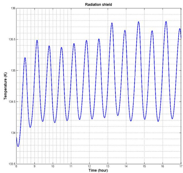
Figure 20. Evolution of the radiation shield temperature
