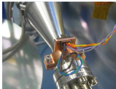
Figure 14. PT100 sensor of the on/off valve
