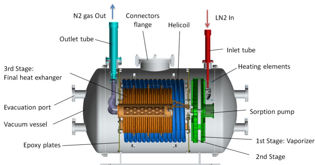
Figure 3. Nitrogen gas preparation unit N2GPU design
