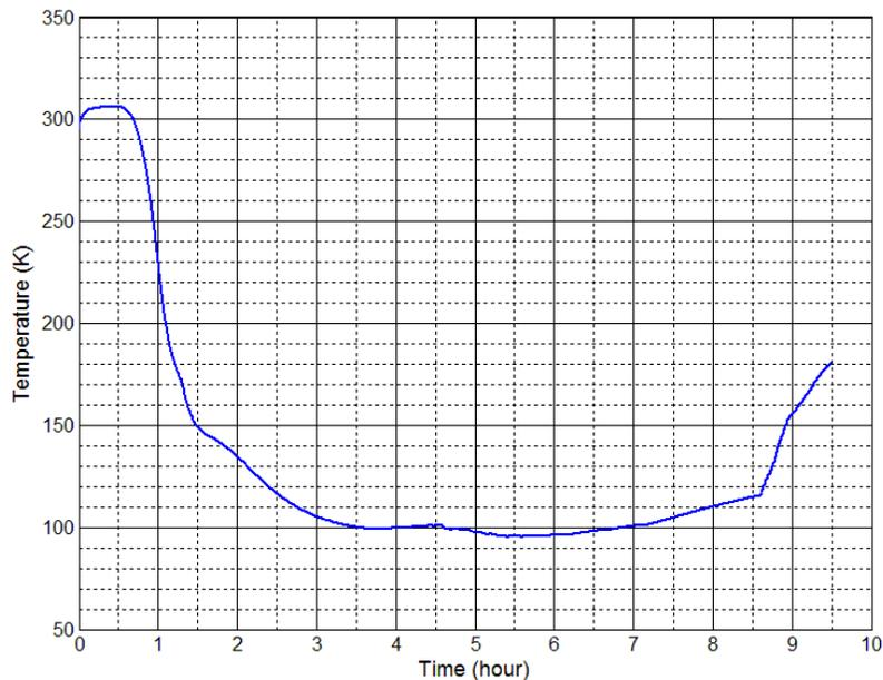
Figure 17. Evolution of the nitrogen gas temperature for test 3
