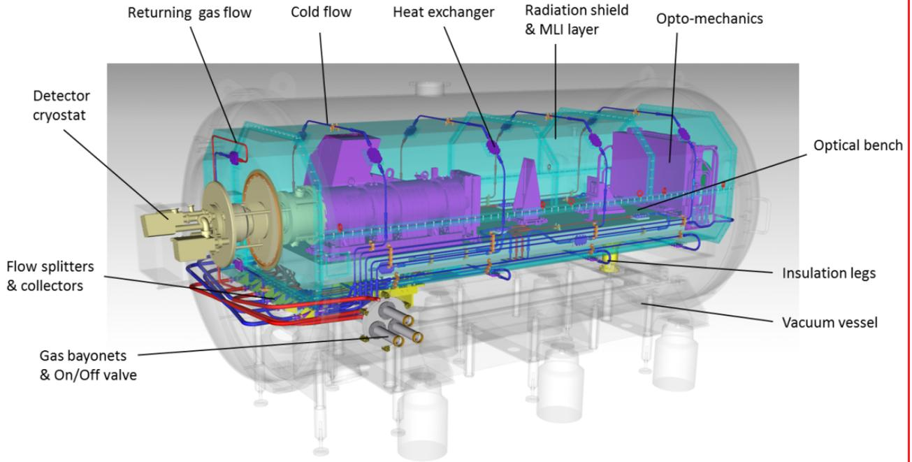
Figure 1. Final design of the NIR channel of CARMENES
