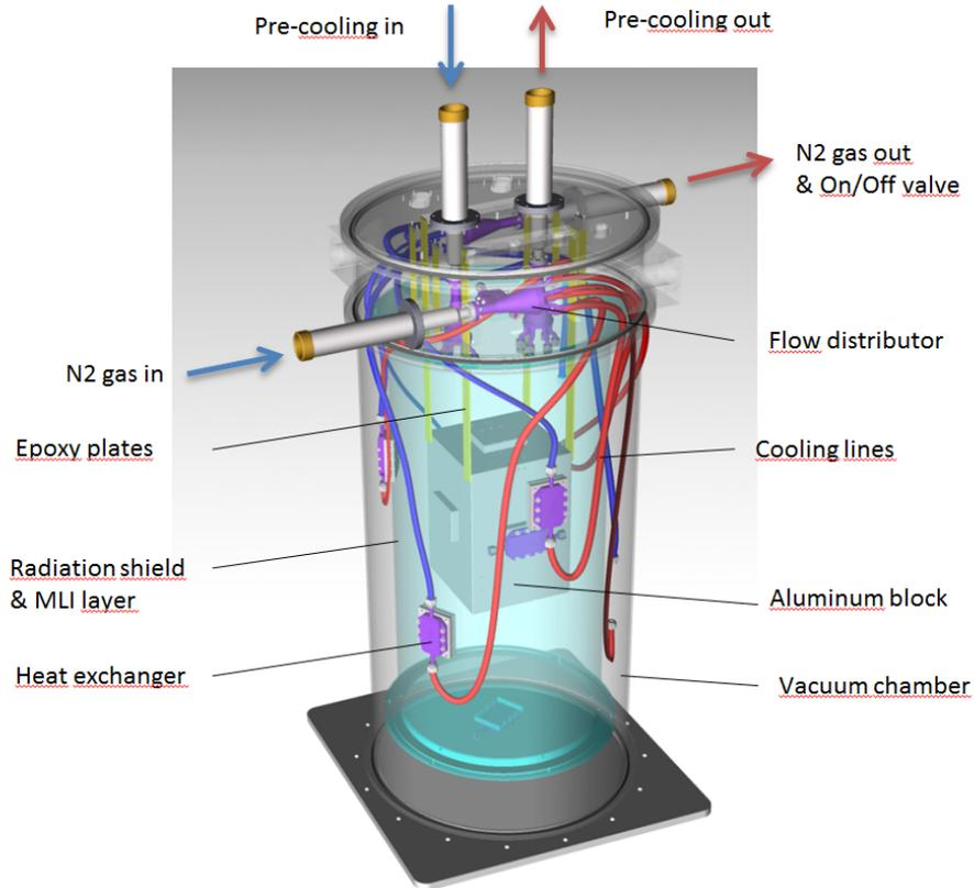
Figure 6. Test facility design
