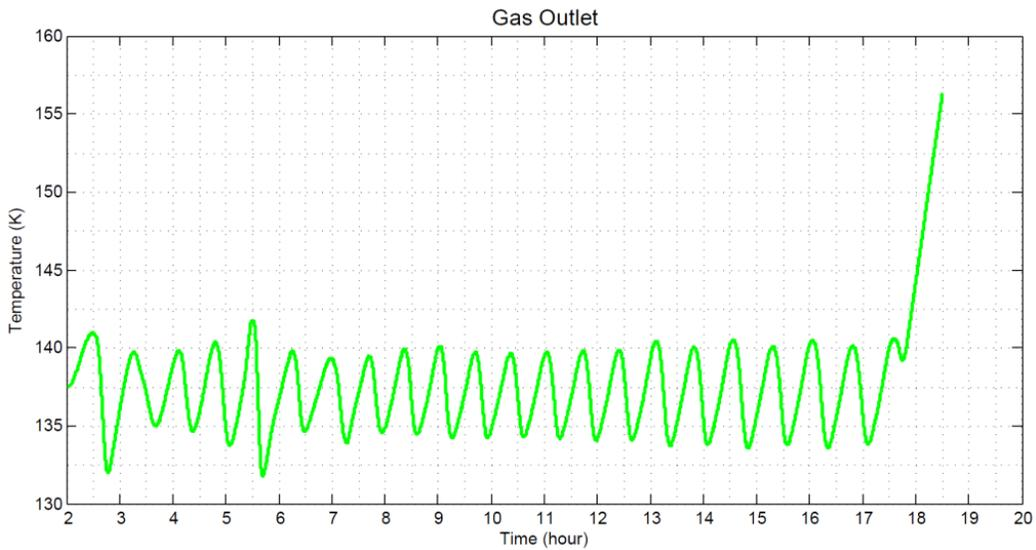
Figure 22. Evolution of the temperature of the on/off valve sensor
