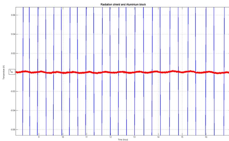
Figure 23. Temperature of the radiation shield and the drift-removed curve of the aluminum block
