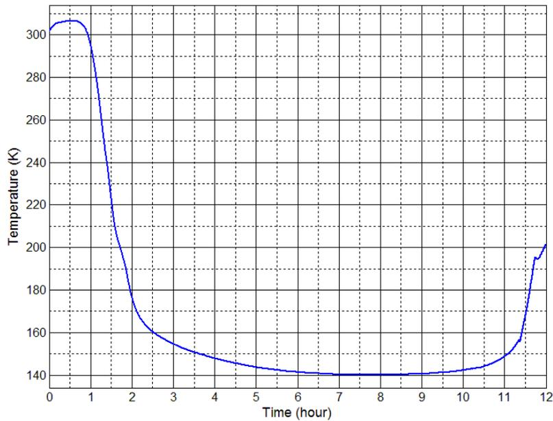
Figure 16. Evolution of the nitrogen gas temperature for test 2
