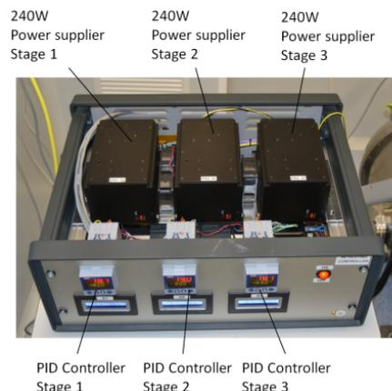
Figure 5. N2GPU PID's controller
