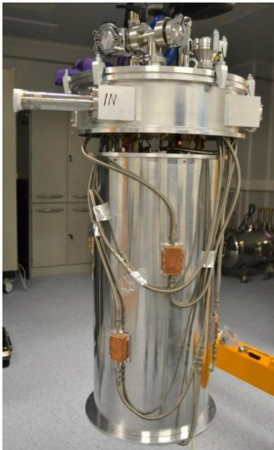
Figure 7. Test facility assembly with the radiation shield
