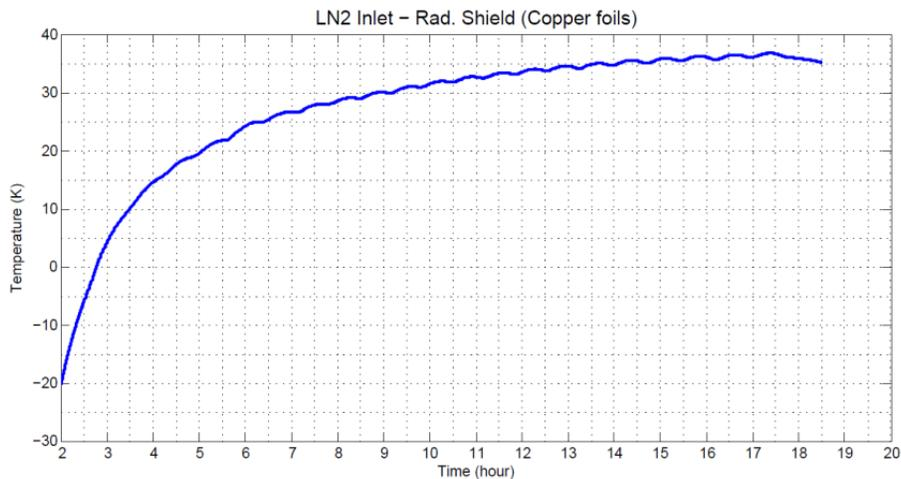
Figure 21. Gap evolution between the temperature of the radiation shield and the pre-cooling inlet bayonet
