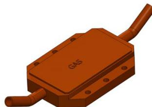
Figure 2. General view of a heat exchanger developed by ESO and extensively used in their instrumentation.
