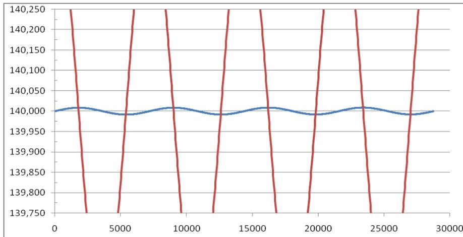
Optical bench temperature oscillation:  $\approx \pm 0.01\text{K}$
