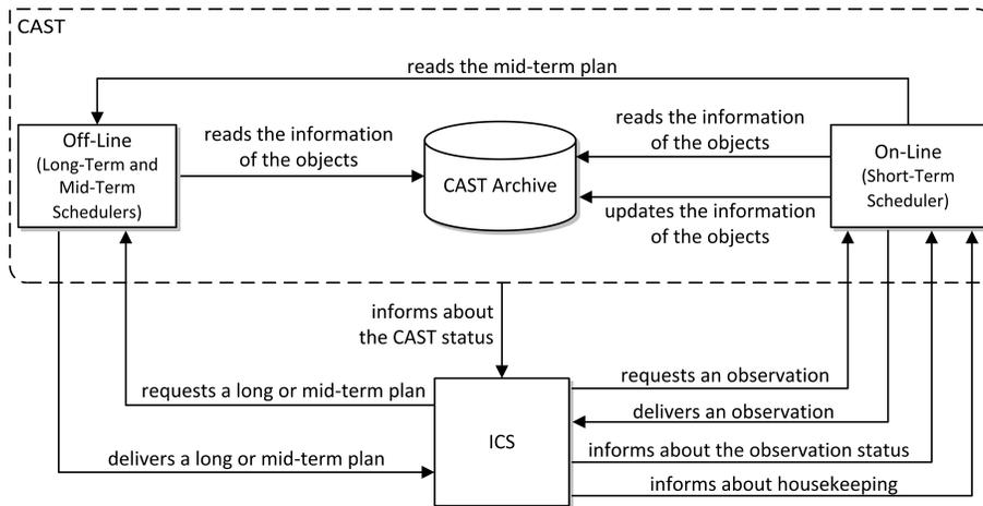
Figure 9: Interactions between CAST and the ICS. The origin of the arrow indicates the element that prompts the action.
