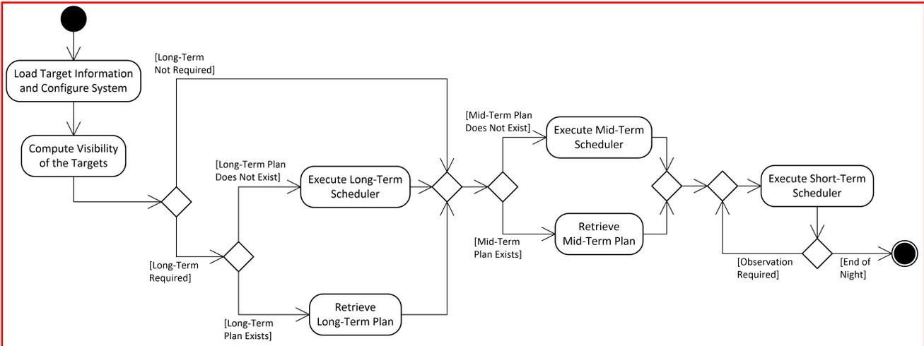
Figure 3: Activity diagram of CAST.
