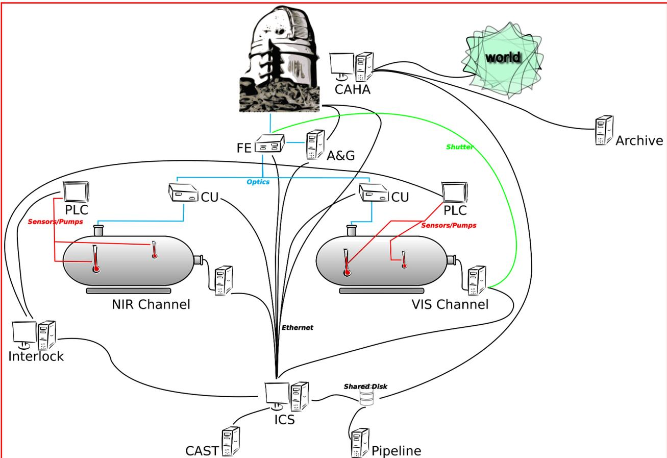
Figure 1: CARMENES System architecture. CU, A&G and FE stand for calibration unit (one for each channel), acquisition and guiding (A&G), and front-end electronics. The PLCs, one set for each channel, are programmable logic controllers.
