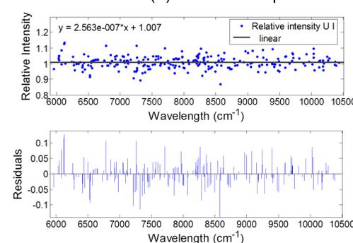
Figure 5. Intensity comparison between HKH0128 and the averaged of all the lamps.
