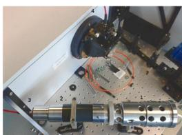
Fig. 2. (1) U-Ne-housing. (2) Optical alignment tool. (3) Fiber input. (4) FTS parallel port.
