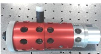
Fig. 1. HCL housing. Numbers indicate the three screw for alignment (1) and three screws for focusing (2).
