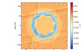
Fig. 1: Overview of the fibers used in CARMENES. CU stands for calibration unit. EM for exposure meter. (left) Measurement of the difference in refractive index of the octagonal part of the science fibers clearly reveals the octagonal core shape and the double cladding structure (top).
