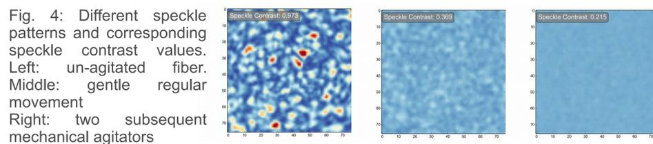
Fig. 4: Different speckle patterns and corresponding speckle contrast values. Left: un-agitated fiber. Middle: gentle regular movement. Right: two subsequent mechanical agitators
