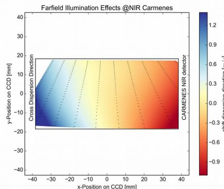
Fig. 3: Spot diagrams with rays of different weights. The weights are indicating the illumination strength of each ray in the pupil plane of the spectrograph. (top) A varying farfield entails a change of the illumination of the pupil plane and therefore a shift of the barycenters on the detector. Expected radial velocity errors for typical farfield variation in the visual and the near infrared (left column).
