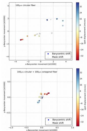
Fig. 2: Barycentric movements of the output of different optical fibers will translate into RV shifts. By combining a circular + octagonal fiber the barycentric shifts for different coupling conditions (simulating a star moving across the fiber) can be reduced significantly (left column). The spot displacement at the entrance of the fiber of  $\pm 40$  micron corresponds to a movement of the star of  $\pm 0.6$  arcsecond on sky.
